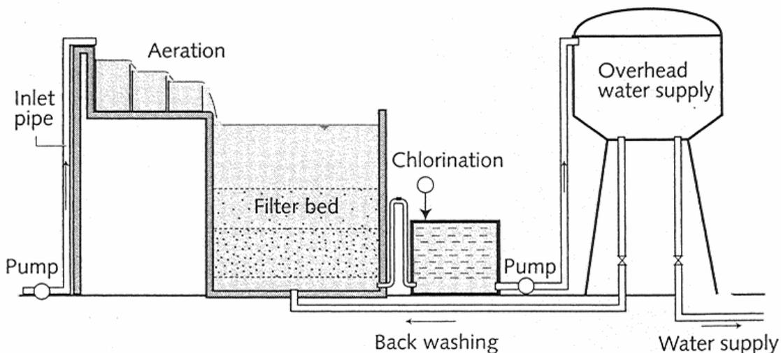
Figure 3. Conventional iron removal treatment unit (Ahsan 2002)
